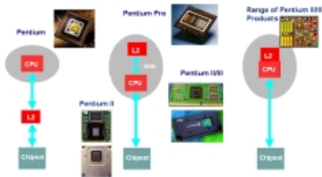
Figure 9: Evolution of the microprocessor and cache architecture from the i486™ microprocessor to the Intel® Pentium® Pro microprocessor
