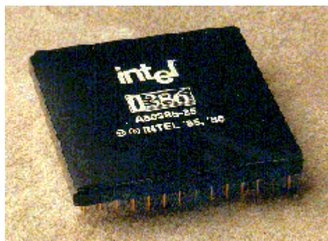
Figure 2: A 132L ceramic PGA package used for the i386™ microprocessor
