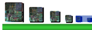
Figure 14: Die shrinks driven by advances in silicon technologies necessitate corresponding improvements in chip-to-package interconnectivity
